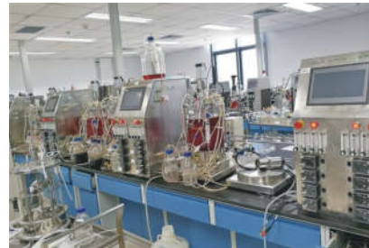
BLBIO-7GJ-4-H Mechanical mixing quadruple glass fermenter (5L)
