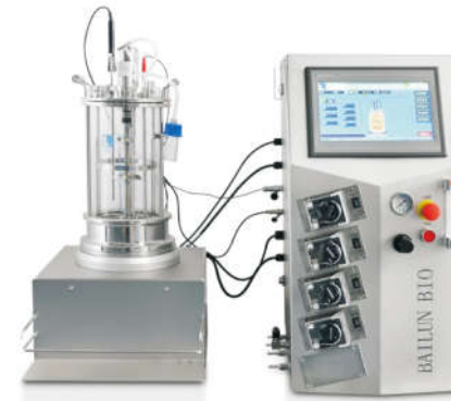
BLBIO-5GC Off-site sterilization magnetic driving glass fermenter (magnetic mixing fermenter)
