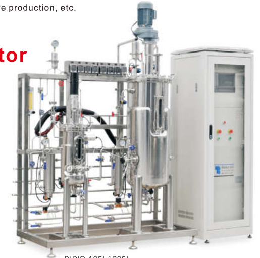
BLBIO-10SJ-100SJ 10L-100L secondary automatic fermenting system
